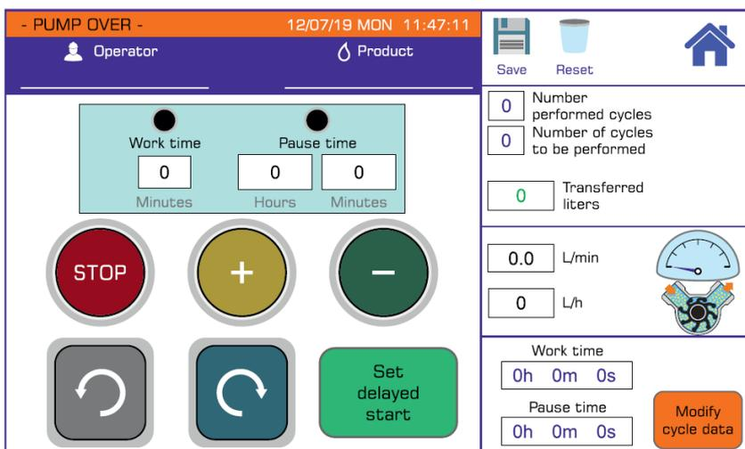
Pump-Over can be achieved by the programming of automatic work/pause cycles as well as pipe emptying operation.
