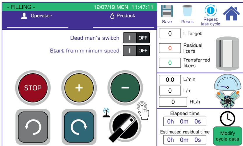
A predetermined batch quantity is entered, the pump is started at the desired speed of operation and, once the target has been reached and the programme completed, the pump is stopped automatically.
