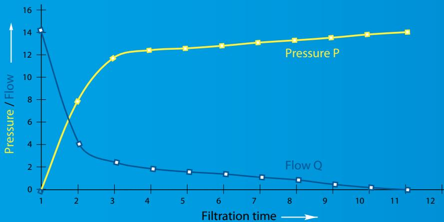
At the beginning of slurry transfer to the filter press the pump operates with high flow but low pressure as the chamber of the filter press is empty.
