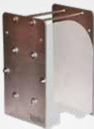
All plastic TF pumps are equipped with stainless steel reinforcement plates to provide better rigidity of the pump making it more robust. To enhance stability even further, the plates are higher than the pump to support the discharge side of the pump. Aluminium pumps are screwed together by means of pinscrews instead of standard screws.
